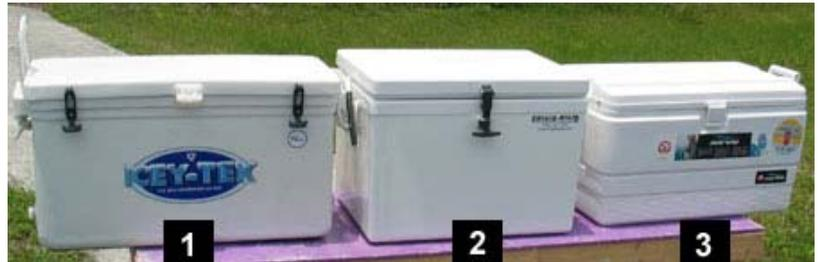
All of the coolers were maintained in the same environmental conditions prior to and throughout the duration of the test. On the first day of the experiment, each of the coolers was filled with 60 pounds of cube ice purchased at a local convenience store. The coolers were kept outside in the sun for about 9-10 hours each day and in a secured warehouse in the evening.
